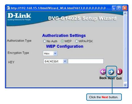
**WEP** is for general use and utilizes a Shared Key between cooperating Wireless devices. WEP encrypts the data portion of each frame transmitted from the wireless adapter using one of the predefined keys. Decryption of the data contained in each packet can only be done if the both the receiver and transmitter have the same shared key.
